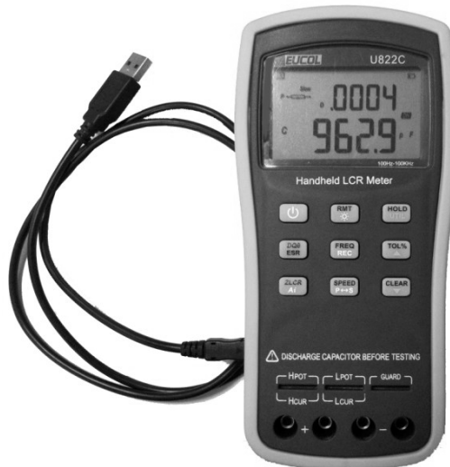
Figure 15- Connection to PC
