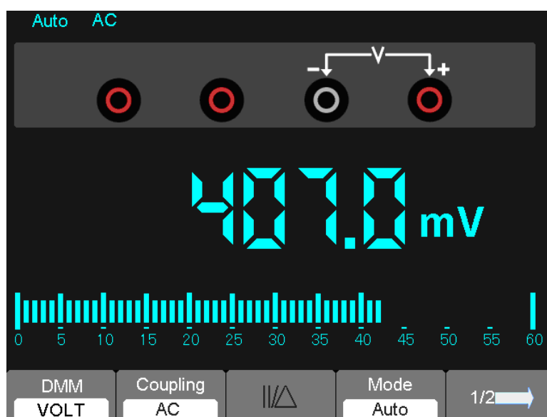
Figure 7-7 AC voltage Measurement
