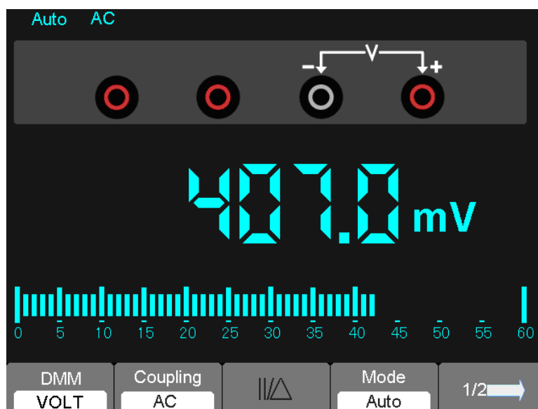
Figure 7-7 AC voltage Measurement
