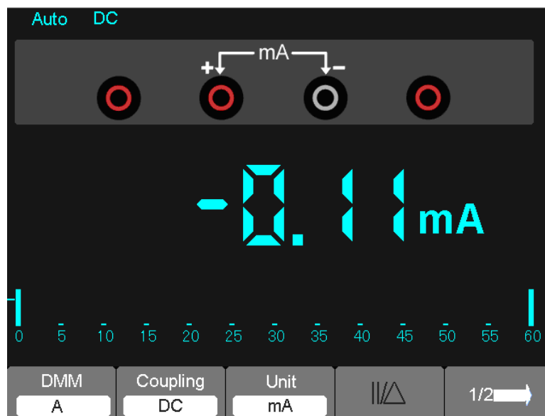
Figure 7-8 DC current Measurement for 600 Measurement
