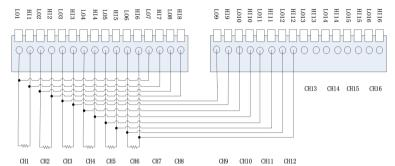
Remarks: [1] To minimize voltage errors, the remote sense connections (CH7,CH8 etc..) should be made as close to the device-under-test (DUT) as possible.
