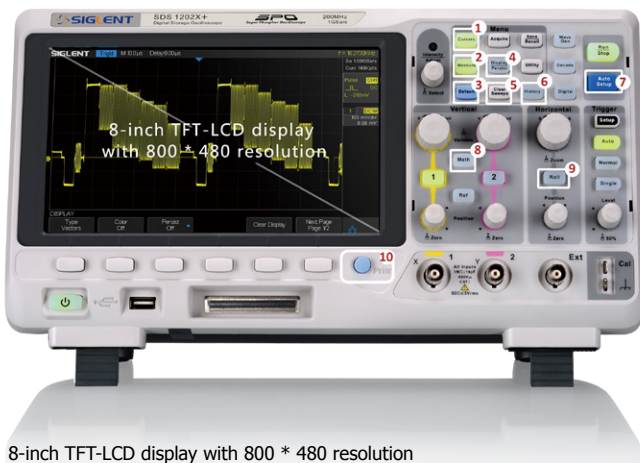
8-inch TFT-LCD display with 800 * 480 resolution
