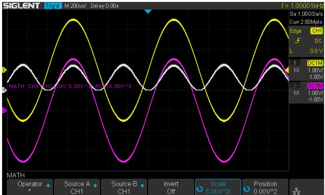
Figure 55 CH1\*CH1 Waveform
