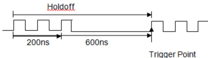
The correct holdoff setting is typically slightly less than one repetition of the waveform. Set the holdoff to this time to generate a unique trigger point for a repetitive waveform. Only edge trigger and serial trigger have a holdoff option. The holdoff time of the oscilloscope is adjustable from 80ns to 1.5s.
