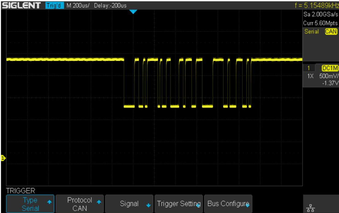
Figure 49 CAN Trigger
