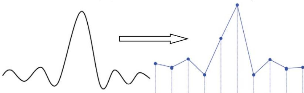
2. **Waveform Confusion:** When the sample rate is lower than twice the actual signal frequency (Nyquist Frequency), the frequency of the waveform rebuilt from the sample data is lower than the actual signal frequency. The most common aliasing effect is the
