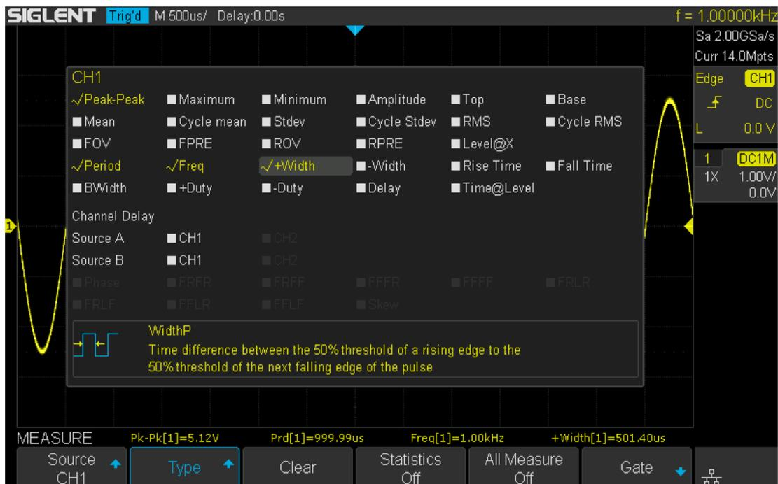
Figure 66 Select the Measurement Parameter
