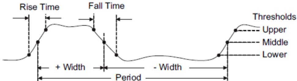
Figure 65 Time Measurements
