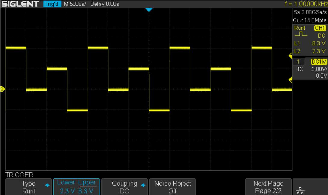
Figure 33 Runt Trigger
