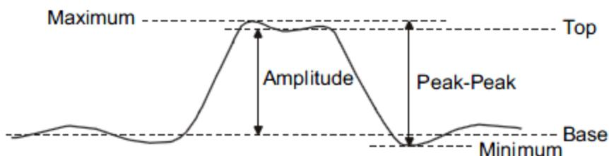
Figure 62 Voltage Measurements
