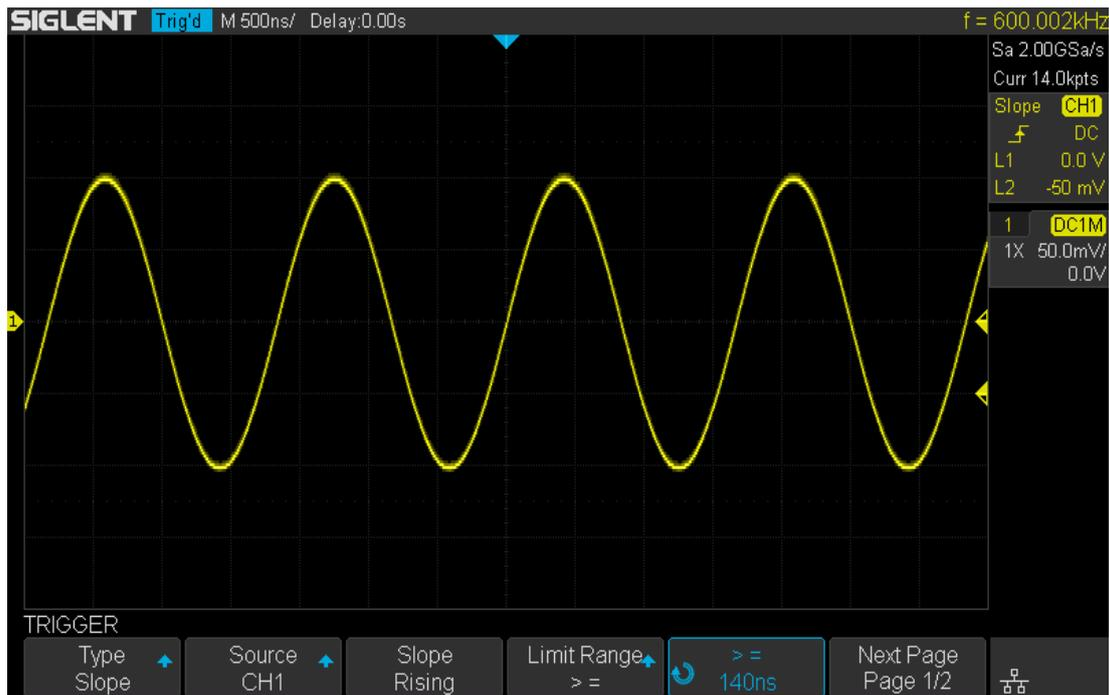
Figure 25 Slope Trigger
