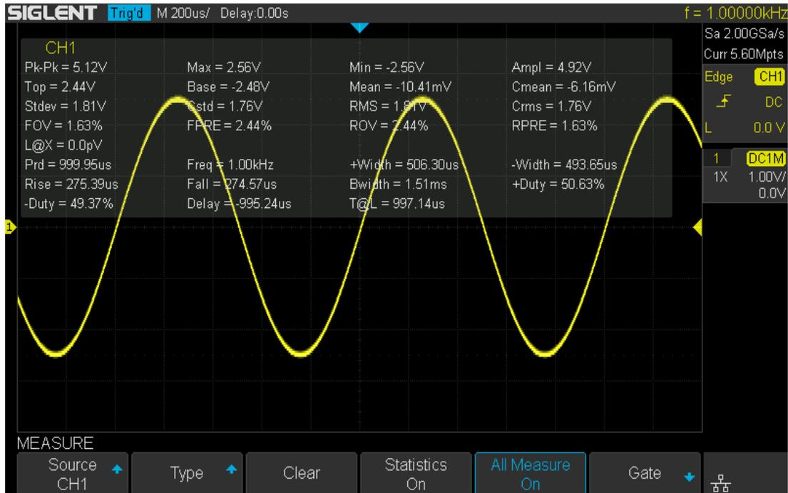
Figure 68 All Parameters Measurement
