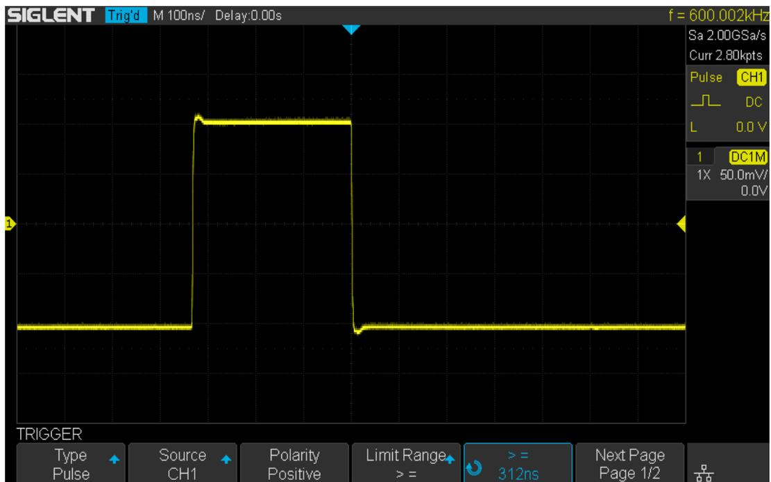
Figure 26 Pulse Trigger
