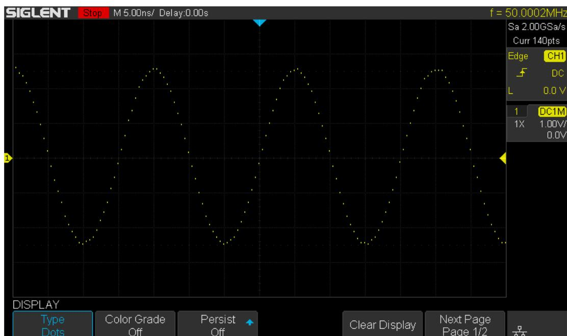
Figure 75 Dots Display
