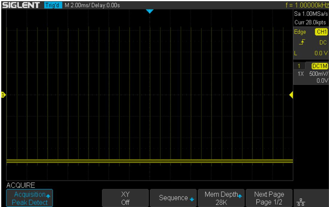
Figure 17 Pulse With 0.01% Duty, Peak Detect Mode
