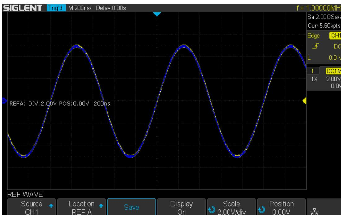
Figure 53 Reference Waveform
