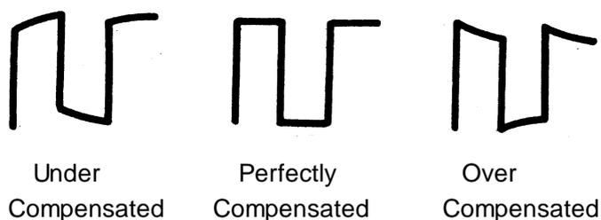
3. Use a nonmetallic driver to adjust the low-frequency compensation adjustment hole on the probe until the waveform displayed is as the “Perfectly compensated” in the figure above.
