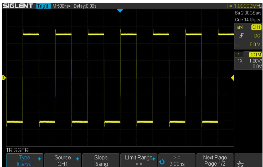
Figure 30 Interval Trigger
