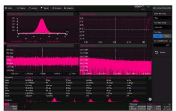
Supports eye diagram and jitter analysis/measurement. It can automatically extract the embedded reference clock from serial data and create the eye diagram. Measurement on multiple eye/jitter parameters is provided. Mask test on eye diagrams is supported
